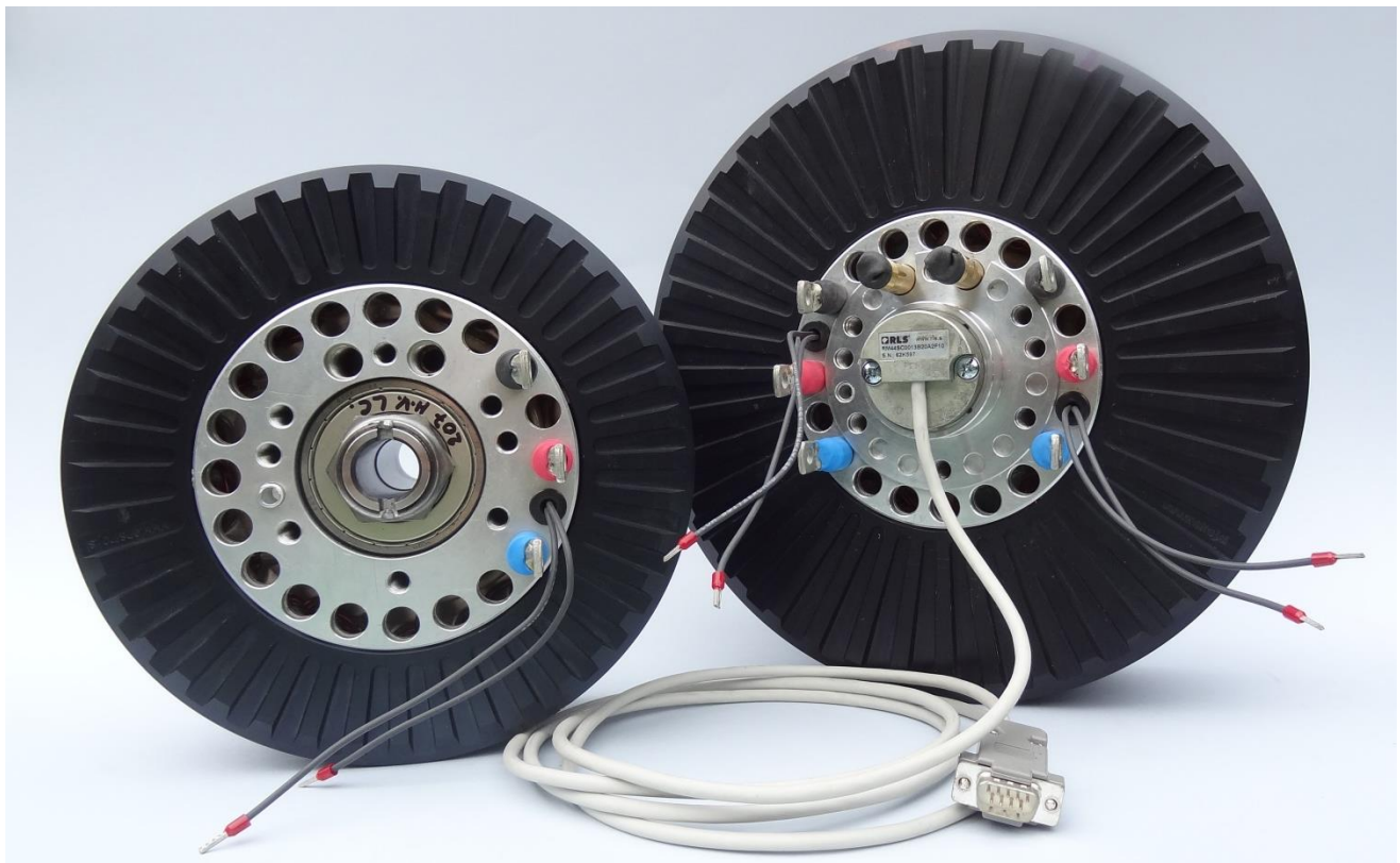
Figure 21: Motor phase connectors – normal (UVW) and doubled (2xUVW)
