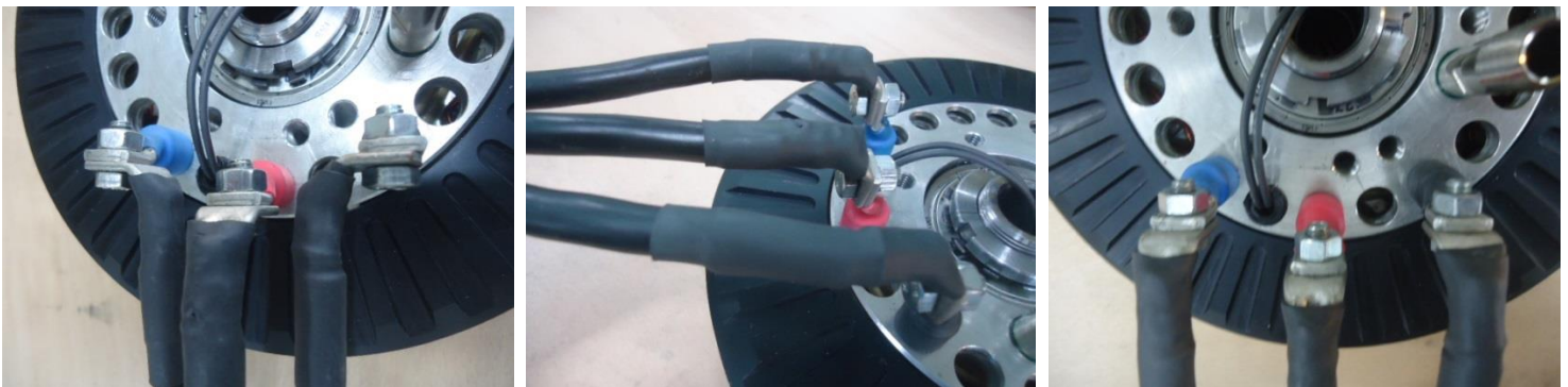
Figure 28: Straight connection of motor phase connectors to controller cables.
