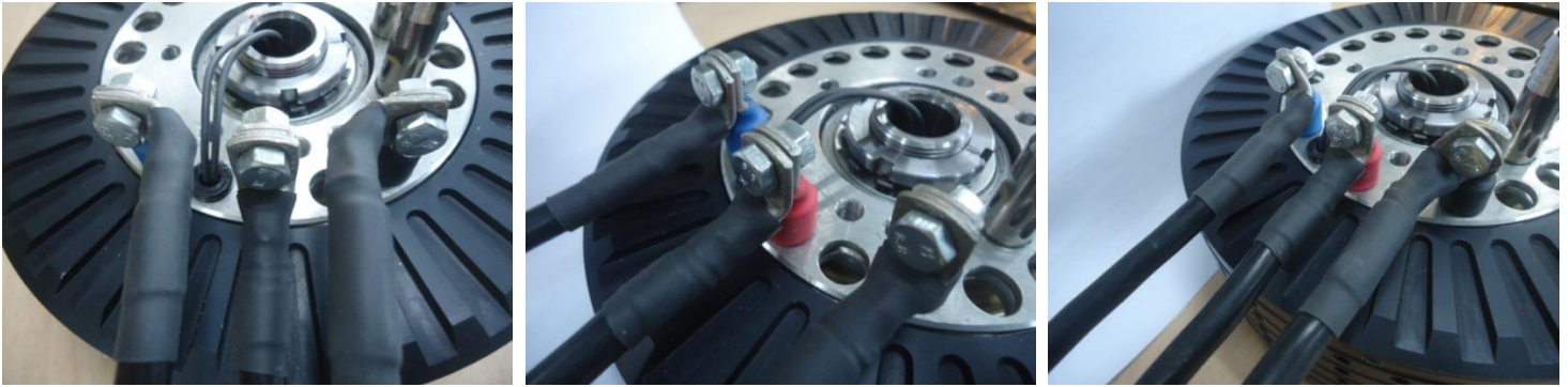
Figure 29: Angular connection of motor connectors to controller cables. Connections must be isolated with shrink hose!
