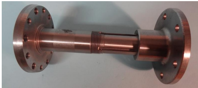
Figure 24: EMRAX TWIN shafts – ESO is mounted in the first motor and FSI on the front side of the second motor
